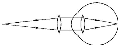
**A convex lens can be used to correct long-sightedness.**
