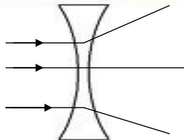
When light rays pass through a convex lens they **come together (converge)**. When light rays pass through a concave lens they **move apart (diverge)**. The more curved a lens is the **greater** the effect on the light rays.
