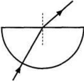
When the angle of incidence is smaller than the critical angle most of the incident light is refracted into the air.
