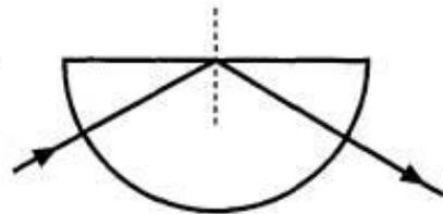
When the incident angle is greater than the critical angle no light is refracted into the air. All light is reflected back into the prism.
