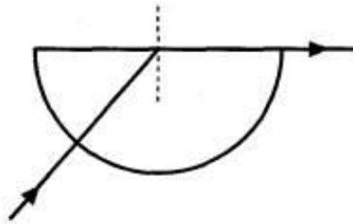
When the incident angle is equal to the critical angle light is refracted into the air at 90 degrees.
