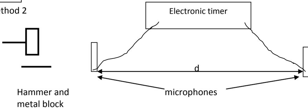
The distance,  $d$ , is measured with a metre stick. The hammer is struck against the block. As the sound reaches the first microphone the timer is started, when it reaches the second microphone the timer is stopped. The equation  $d = vt$  is used to calculate the speed again. This is a much more accurate method.
