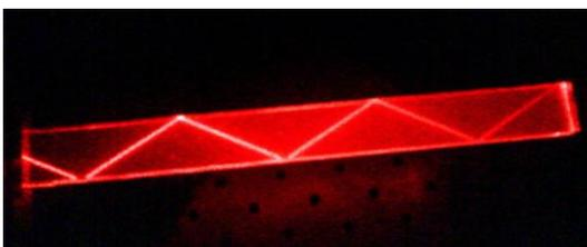
Total internal reflection is used in optical fibres. Optical fibres can be used for communication or in medical applications to allow doctors to see into the body. One bundle of fibres carries light into the body whilst another carries the light back out of the body. This instrument is known as an **endoscope**.
